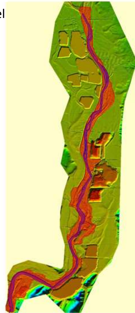
Figure 6 A) Location of the flow model grid over the existing topographic surface. B) The location of the short reach used in the morphodynamic simulations. C) The location roughness polygons used to define the un-vegetated channel (blue), the vegetated channel (red).
