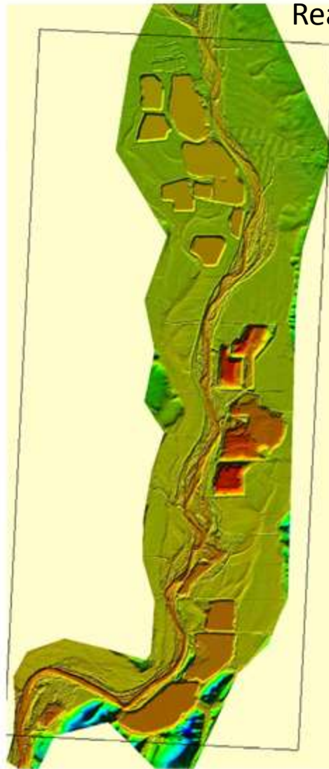
Figure 6 A) Location of the flow model grid over the existing topographic surface. B) The location of the short reach used in the morphodynamic simulations. C) The location roughness polygons used to define the un-vegetated channel (blue), the vegetated channel (red).
