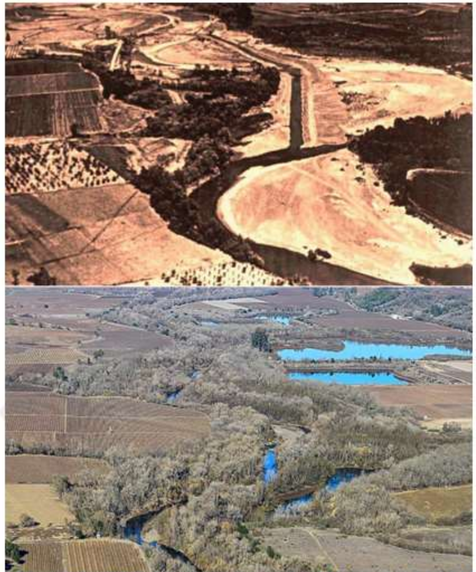
Figure 4.1.3. Changes in the Middle Reach of the Russian River. The upper photo shows the Middle Reach in the mid-1950's (Press Democrat), and the lower photo is the same area in December 2013). The wide meanders were dredged, replacing the sinuous channel with a straightened alignment and then the gravel bars were mined. The channel was dredged 50-60 feet deep which drove incision along with its shorter and steeper path. Once incised, agriculture encroached tightly on the river bank, which has levees along most of its length along the Middle Reach channel. Photo by Brian Ower, NOAA Fisheries.
