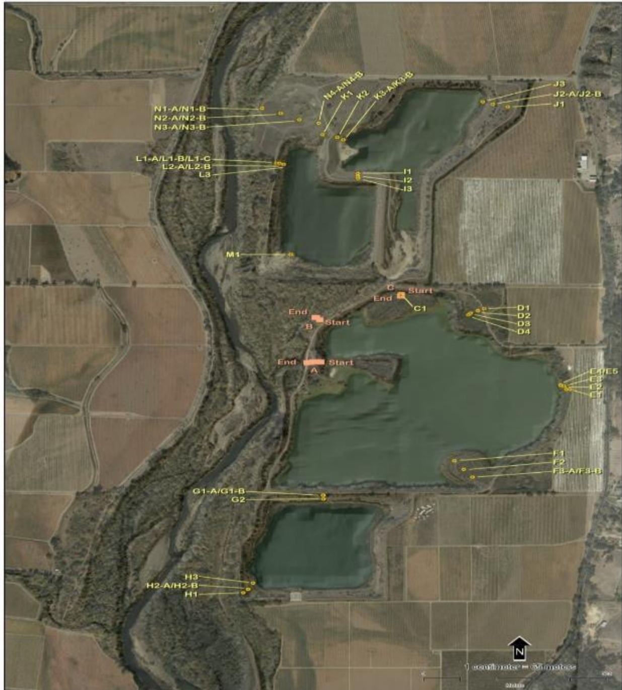
Figure 4.3.11. Terrestrial sediment sampling locations around the Hanson ponds. Trench and test pits locations for soil samples were taken from the 45 locations shown below for characterization of the Hanson site levees and upland soils to characterize grain size distribution and stratigraphy. Sampling locations and sample identifiers are referenced in Table 4.3.1.
