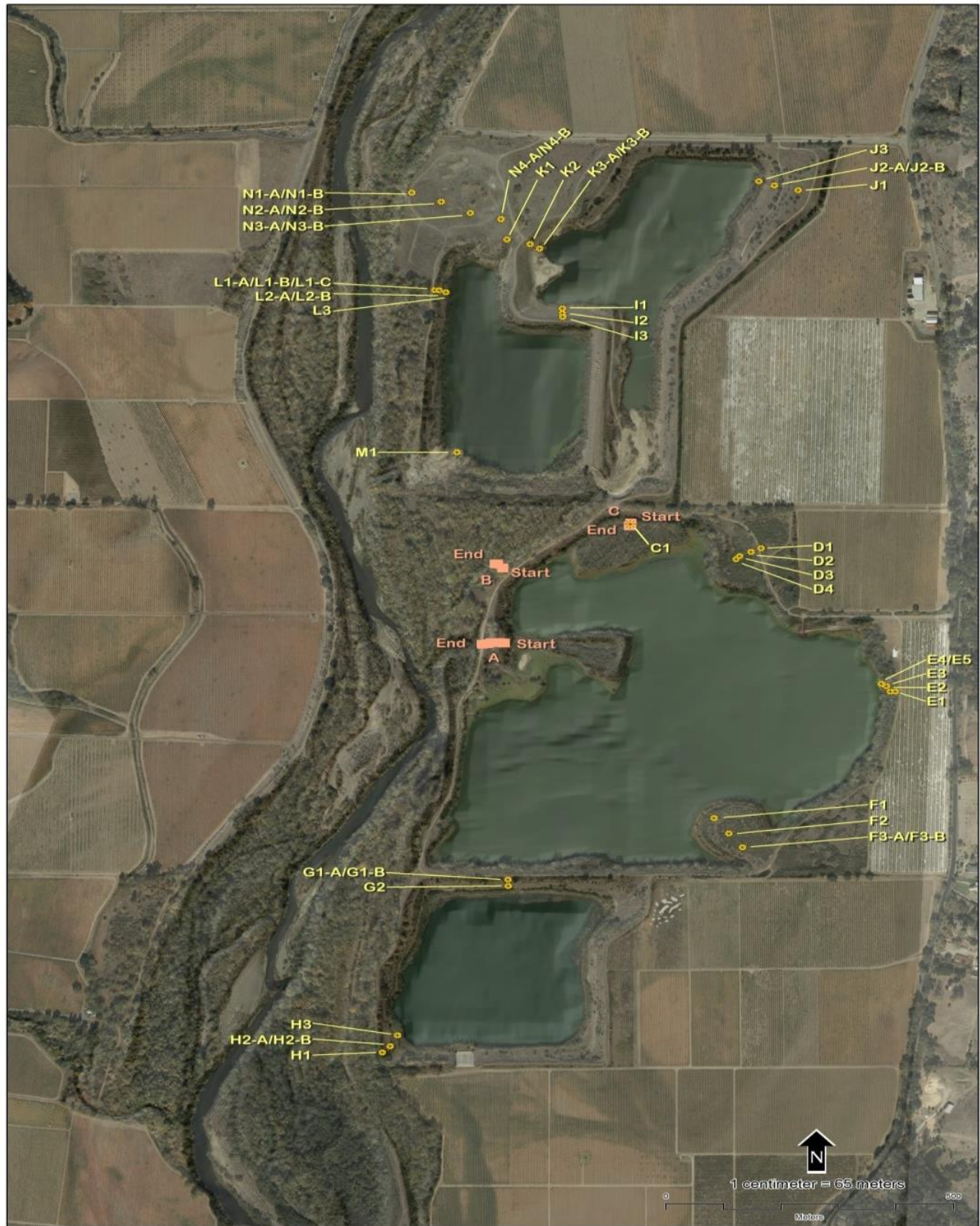
Figure 3.4. Terrestrial sediment sampling locations around the Hanson ponds. Trench and test pit locations for 45 samples for Hanson site grain size distribution and soil stratigraphy characterization.
