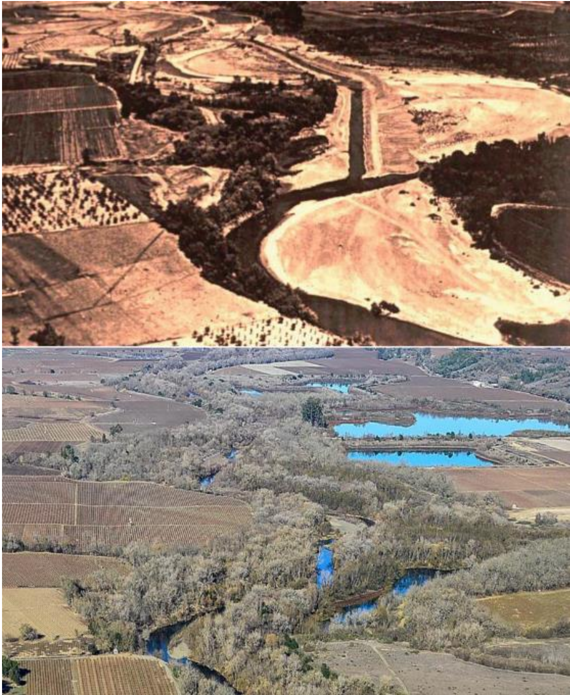
Figure 4.1.3. Changes in the Middle Reach of the Russian River. The upper photo shows the Middle Reach in the mid-1950s (Press Democrat), and the lower photo is the same area in December 2013. The wide meanders were dredged, replacing the sinuous channel with a straightened alignment and then the gravel bars were mined. The channel was dredged 50-60 feet deep which drove incision along with its shorter and steeper path. Once incised, agriculture encroached tightly on the river banks, which have levees along most of the length of the Middle Reach channel. Photo by Brian Cluer, NMFS.
