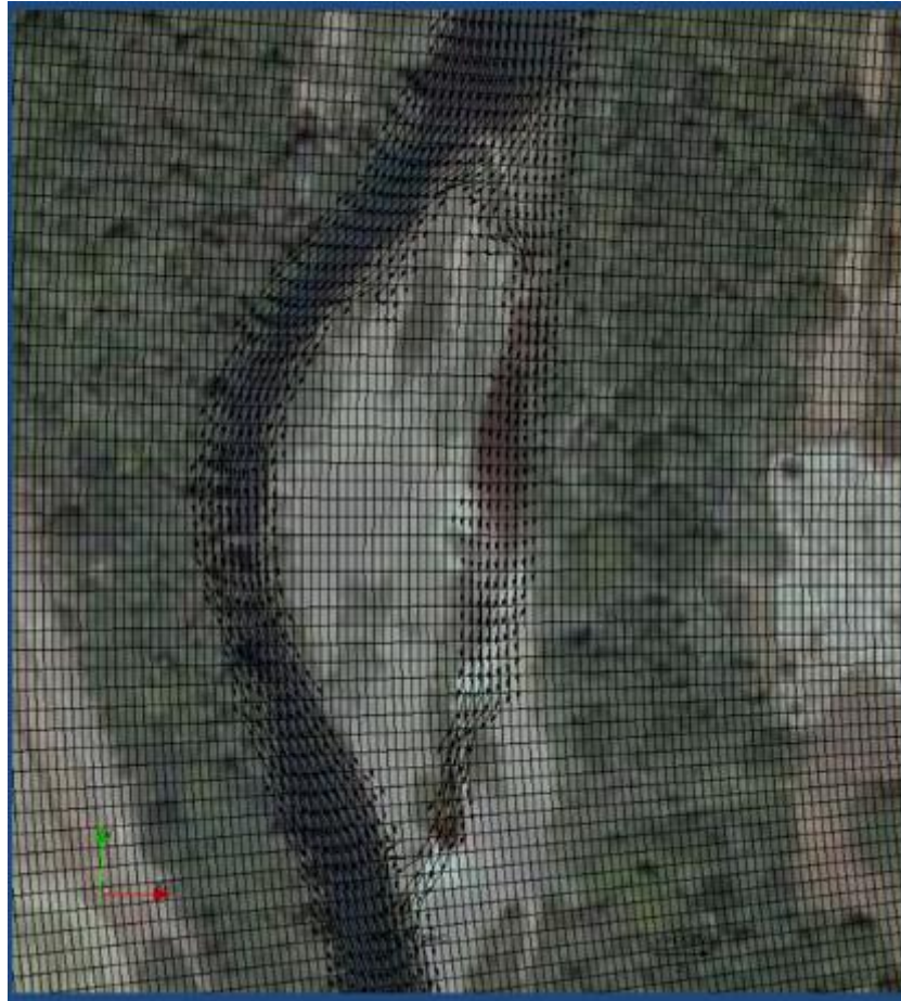
Figure 4.3.8. Example of short section of the river channel bathymetry integrated into grid mesh of LiDAR derived topography of the Middle Reach floodplain.
