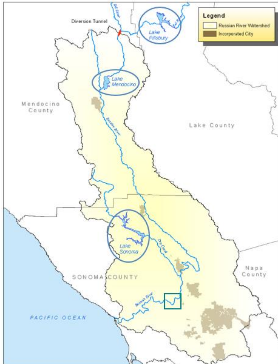
Figure 4.2.7. Sonoma County Water Agency reservoirs and infrastructure. The system has three reservoirs: Lake Pillsbury in the Eel River watershed, Lake Mendocino on the East Fork Russian River, and Lake Sonoma on Dry Creek. Additional system infrastructure includes the Potter Valley diversion tunnel for diversion of Eel River water to the East Fork Russian above Lake Mendocino, and the Wohler/Mirabel pumping station in the lower river at the lower end of the study reach.
